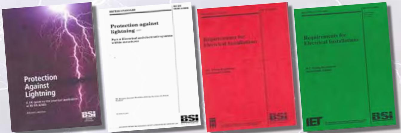
**BS6651:1999 Annex C** - UK Standard Prior to August 2008 -The BSI “Code of Practice for Protection Against Lightning” provides general advice on the protection of electronic equipment, and was replaced in August 2008 by **BS EN 62305-1 to BS EN 62305-5:2006**, although as BS6651:1999 is so well established, it is probable that it will still be referred to as a reference source.
